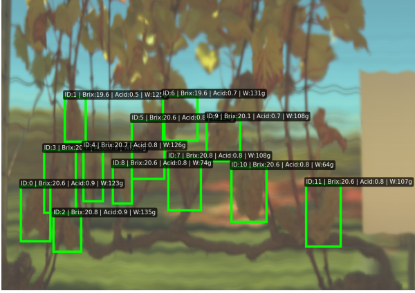
Fig. 6: Visualization of the integrated system’s output on a single hyperspectral scan captured by the robotic platform. The YOLO-based module detects individual grape bunches (green bounding boxes). For each detected bunch, the system predicts and displays its unique identifier (ID), estimated weight (W), and the average predicted quality parameters (Brix and Acidity) derived from the LISA framework. This demonstrates the system’s ability to generate rich, spatially-resolved data points in a complex, in-field environment, which can then be used to create comprehensive vineyard maps.
